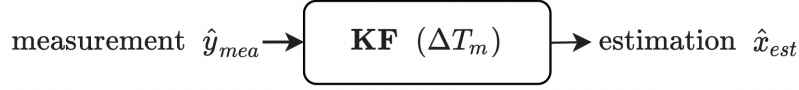
Figure 6.1: The diagram of the linear estimator. ‘KF’ represents Kalman filter which is implemented at measurement sampling time \Delta T_m . The input is measurement \hat{y}_{mea} and the output is estimation \hat{x}_{est} , according to (6.4).
