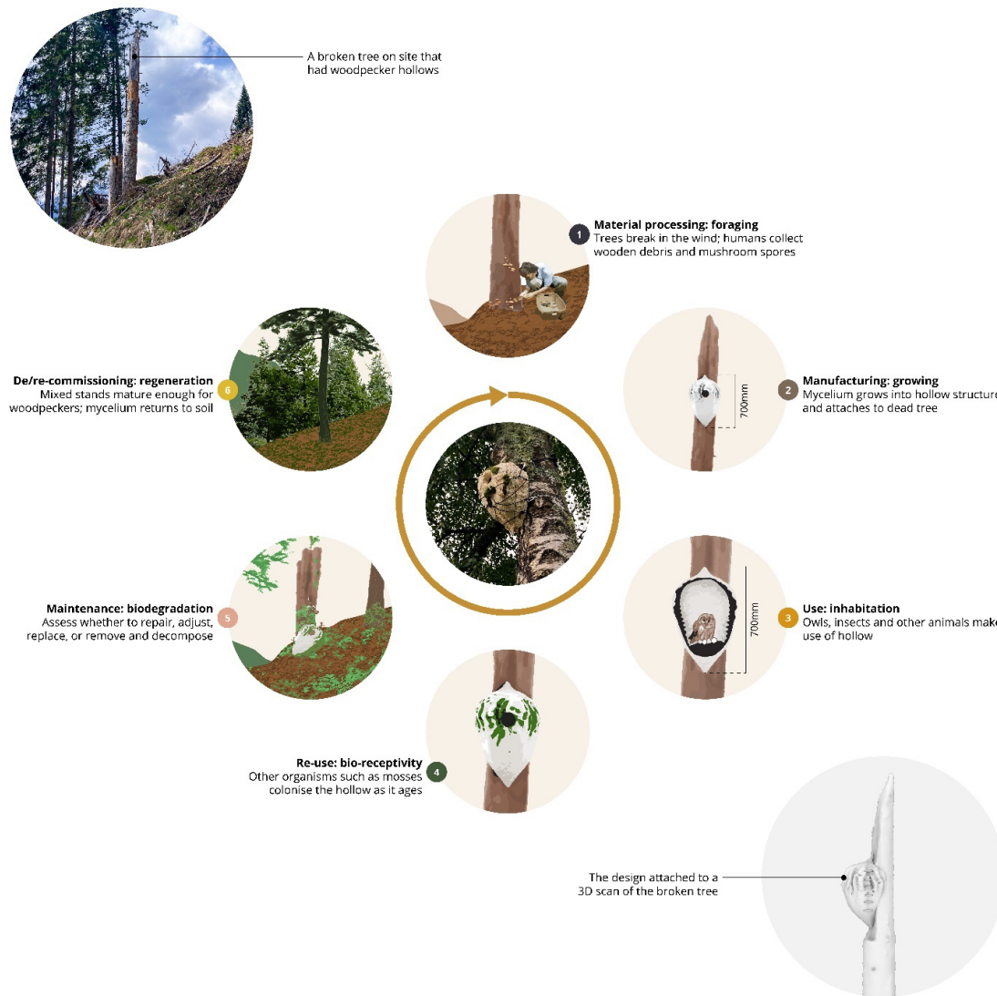
Figure 2. An artificial hollow design that implements a lifecycle approach, proposing to reinstate nesting opportunities on dead trees that had hollows before breaking in a large storm. Image by the authors.
