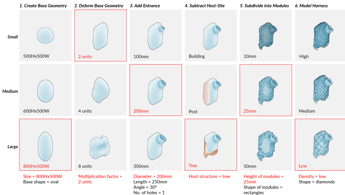
Figure 3. The search space for form-finding and parametric adjustments. Columns: steps generating geometry. Top row: adjustable parameters. Grey rows: examples of options. Red frames: chosen options. Image by the authors.
